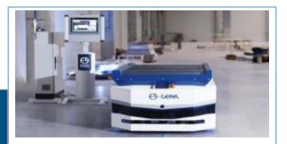
An automated guided vehicle or automatic guided vehicle (AGV), also called autonomous mobile robot (AMR), is a portable robot that follows along marked long lines or wires on the floor, or uses radio waves, vision cameras, magnets, or lasers for navigation. They are most often used in industrial applications to transport heavy materials around a large industrial building, such as a factory or warehouse.
