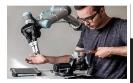
A Cobot, or collaborative robot, is a robot intended for direct human robot interaction within a shared space, or where humans and robots are in close proximity. Cobot applications contrast with traditional industrial robot applications in which robots are isolated from human contact.
