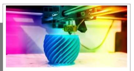
Additive manufacturing (AM) or additive layer manufacturing (ALM) is the industrial production name for 3D printing, a computer controlled process that creates three dimensional objects by depositing materials, usually in layers.
